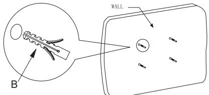
Use the wall plate as a template to drill four holes of dia. 8 mm and 50 mm depth in the wall. Then wedge four plastic anchors into the holes.
