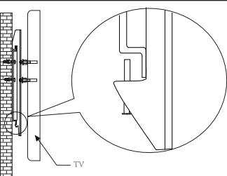
Fix the two bolts under the monitor brackets inside of the wall plate and then screw them down.
