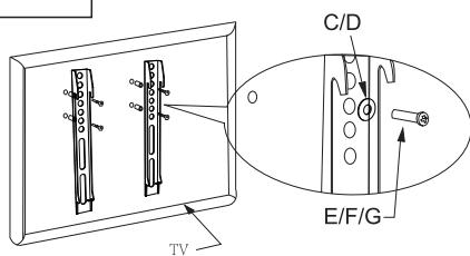
Install the monitor brackets onto the back of the panel TV; screw two bolts into the holes in the back of the panel TV to install each monitor bracket. Make sure the distance from each bracket to the top of the panel TV is equal, and also as center as possible. The parts shall be selected according to the dimensions of the holes in the back of the panel TV.
