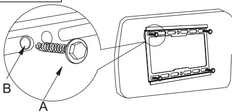
Install the wall plate. Put the wall plate on the wall, and then screw four lag bolts into each plastic concrete anchor through metal washer to fix the lag bolt, the plastic concrete anchor and the wall.
